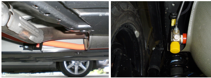
Figure 21: View on the underbody of the vehicle, a. High voltage power cable, b. Gas tank
