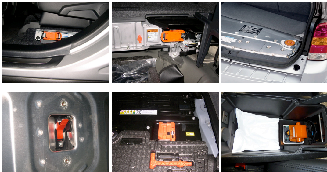
Figure 15: Examples for different service disconnect switches.
