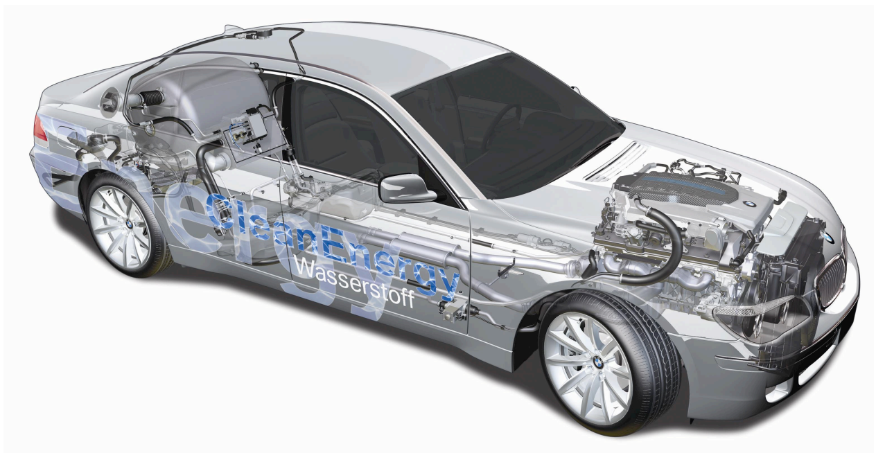
Figure 16: BMW Hydrogen7 test vehicle with hydrogen propulsion. On this vehicle hydrogen will be stored liquefied at -253 °C and burned in an internal combustion engine (courtesy of: BMW).
