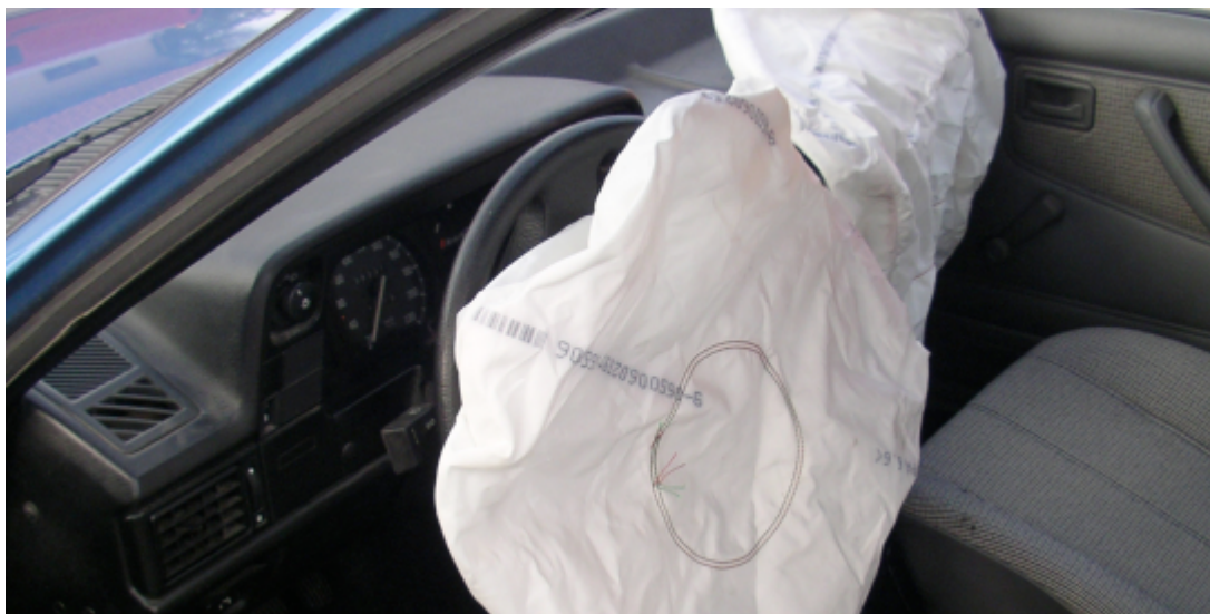
Figure 34: Retrofitted deployed driver and passenger airbags
