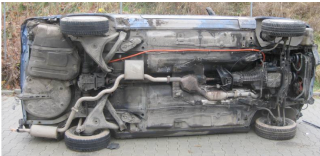
Figure 36: Retrofitted high voltage power cable on the underbody of a vehicle
