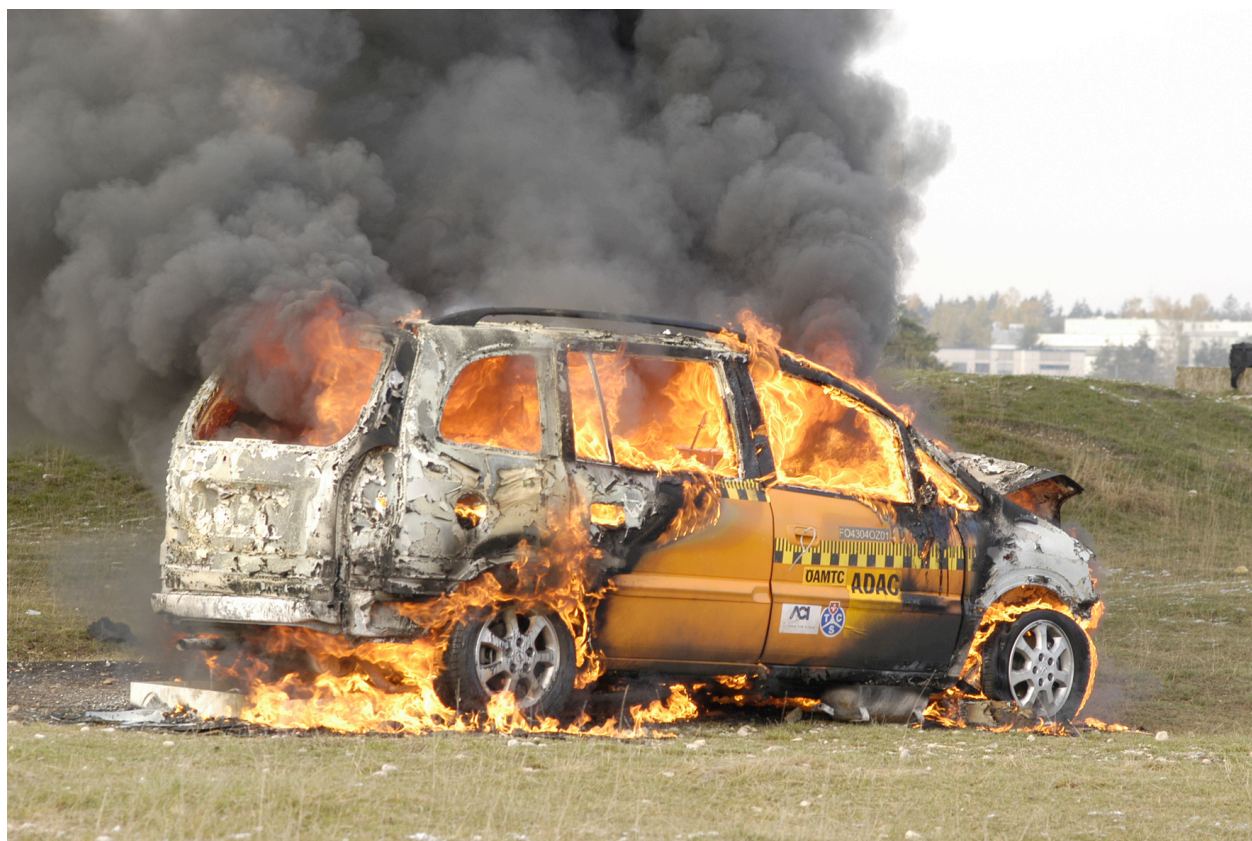
Figure 4: Burn test conducted with a CNG powered vehicle. To avoid an explosion of the CNG tank, pressure relief devices mounted on every tank will vent the CNG in case of exposure to high temperatures (courtesy of ADAC).
