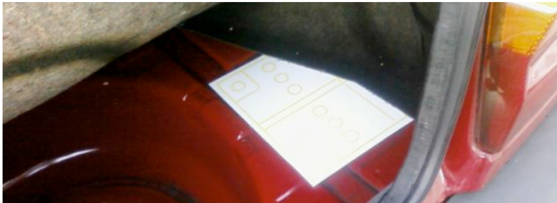
Figure 35: Battery-Dummy in the trunk of a vehicle
