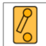
Service/Emergency disconnect switch
