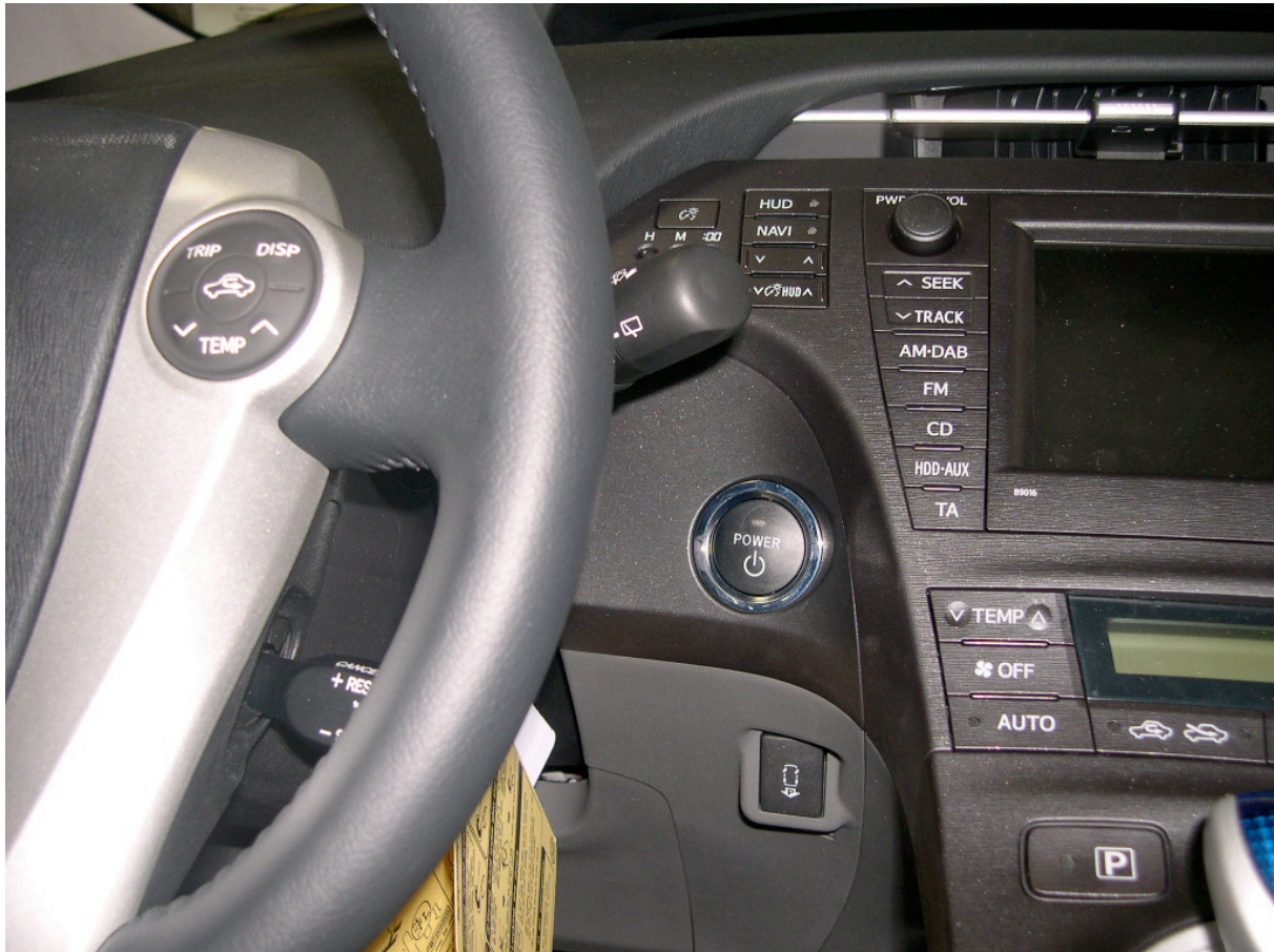
Figure 27: Start/stop-button, shown on a Toyota Prius
