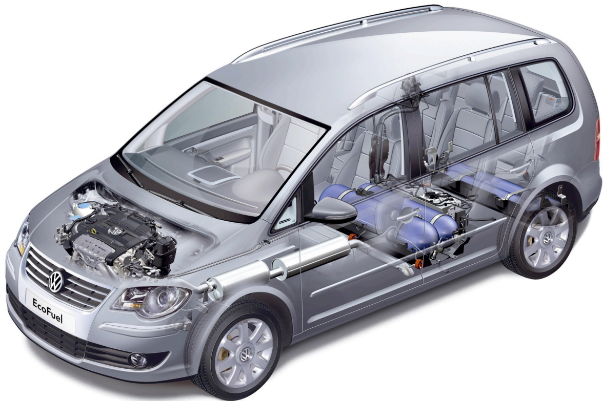
Figure 1: CNG powered vehicle, Volkswagen Touran Ecofuel (Courtesy of Volkswagen AG)
