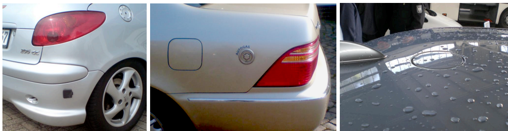
Figure 23: Examples for additional filler caps and uncommon openings.
