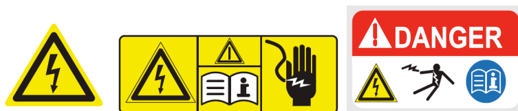
Figure 13: Identification label for high voltage components
