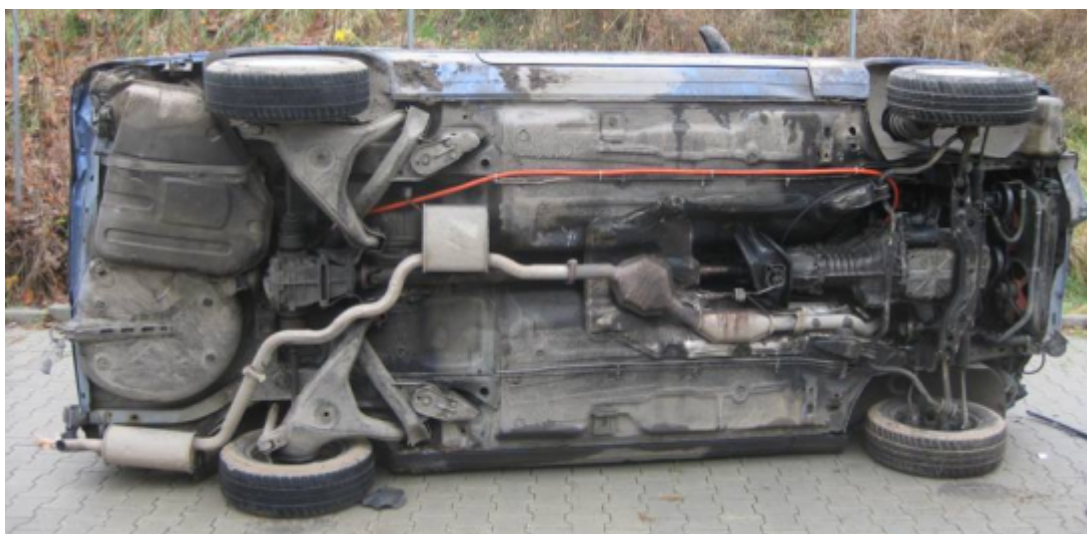
Figure 12: Simulated high voltage power cable on the underbody of a vehicle
