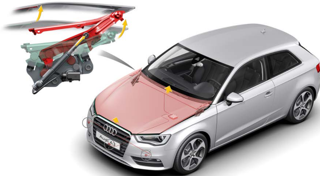
Figure 21: Pedestrian Protection System shown on an Audi A3. Sensors in the front bumper are able to detect a collision with a pedestrian. On detection two pyrotechnically released pistons will lift the rear edge of the hood. This increases the clearance between the hood and engine parts. (Courtesy of Audi)
