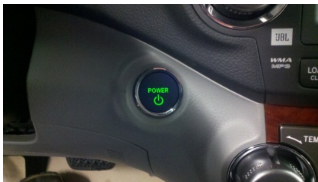
Figure 3: Ignition button on a 2012 Toyota Highlander Hybrid. These will be found on many vehicles, not just alternative power vehicles.
