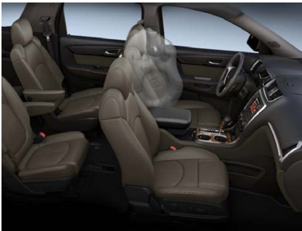
Figure 16: Front center airbag shown on a GMC Acadia. (Courtesy of GM)
