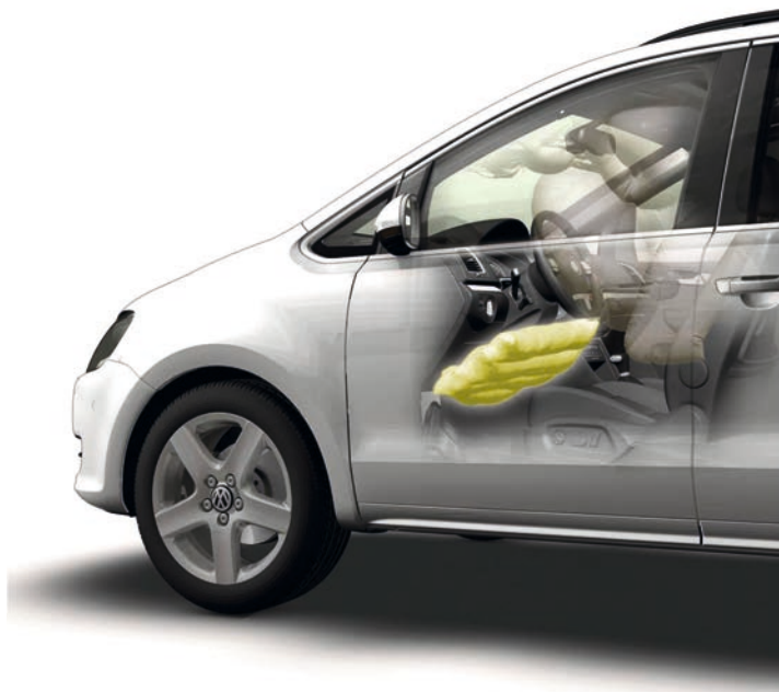
Figure 9: Drivers side knee airbag deploying from the lower dashboard area shown on a Volkswagen Sharan. (Courtesy of Volkswagen)
