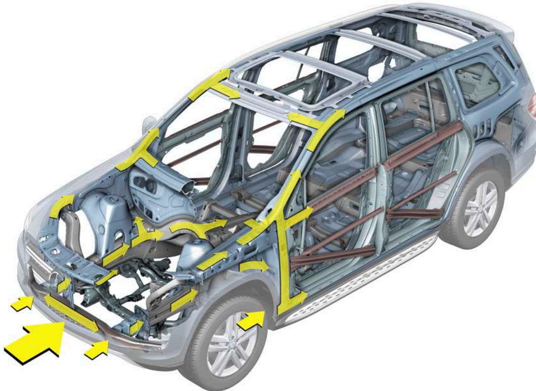
Figure 3: Body structure of a Mercedes-Benz GL-Class. The arrows indicate the load paths in the case of a frontal collision. The front-end assembly is designed as a crumple zone and absorbs crash energy. The safety cell should maintain its integrity as long as possible. (Courtesy of Daimler)
