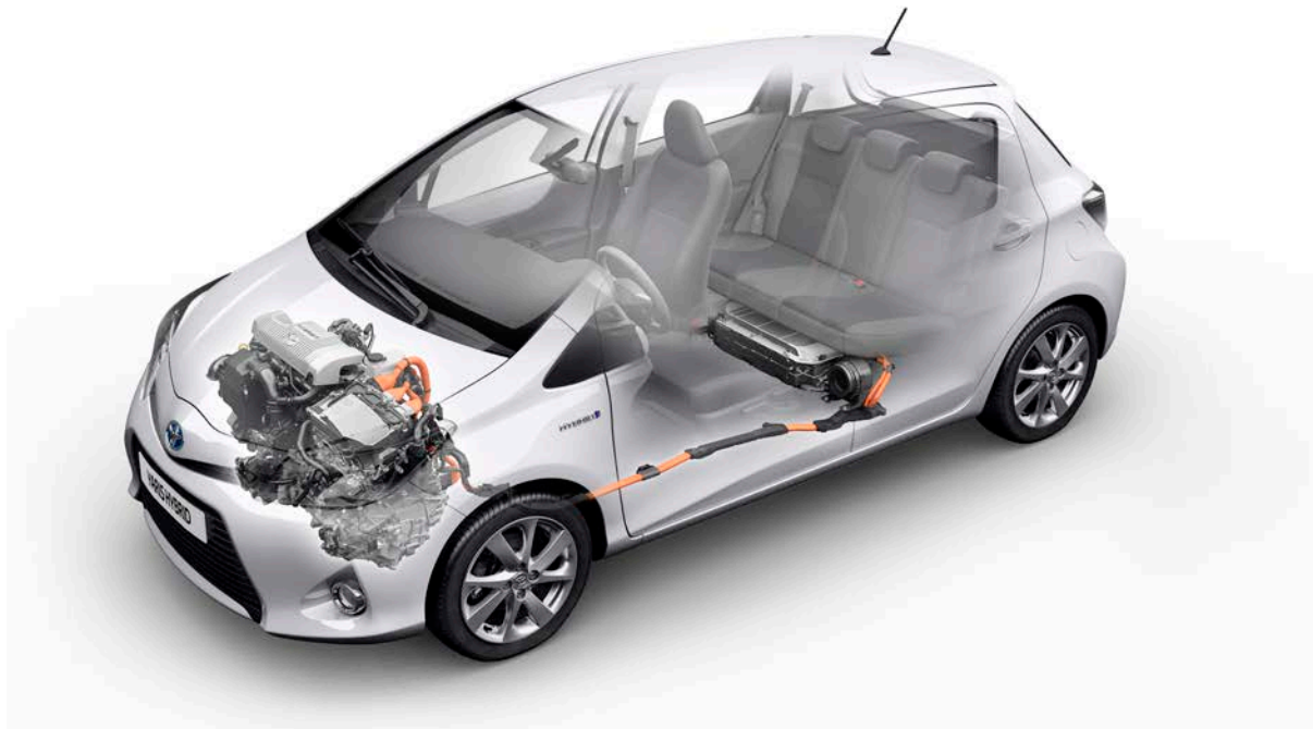
Figure 46: The image of this Toyota Yaris Hybrid clearly shows the location of high-voltage system components. The high voltage battery is located under the rear seat. Orange high voltage cables are routed under the floor of the vehicle to the engine compartment where they are connected to the electric motors and other high-voltage components. (Courtesy of Toyota).
