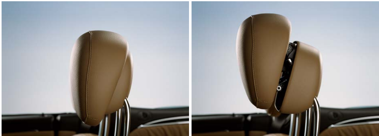
Figure 17: Daimler's Neck-Pro whiplash protection system reduces the clearance between the occupant's head and the headrest in order to avoid hyperextension of the head. (Courtesy of Daimler)
