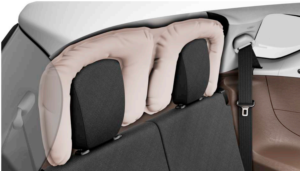
Figure 19: Rear curtain airbag shown on a Toyota/Scion iQ. (Courtesy of Toyota)
