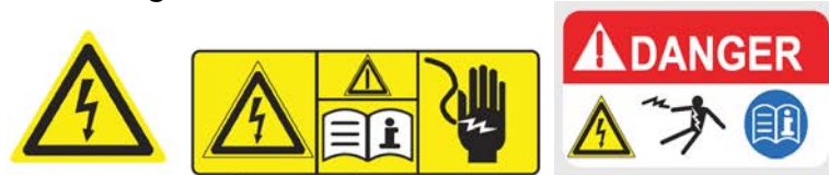
Figure 47: Identification label for high voltage components
