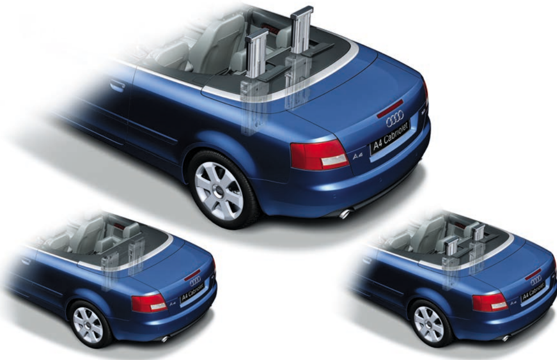
Figure 43: Rollover protection system of an Audi A4 convertible. The two automatic roll bars deploy behind the left and right rear seat. (Courtesy of Audi)
