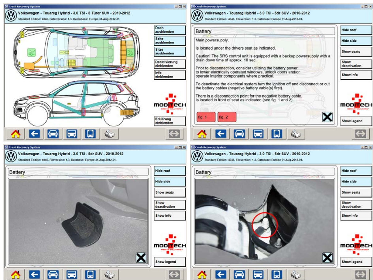
Figure 3: The 12 Volt battery of this Volkswagen Touareg Hybrid is located under the driver's seat. The negative battery cable can be disconnected from the vehicles body on the ground point in front of the driver's seat. This ground point is accessible through a flap in the carpet. The Crash Recovery System contains all information for the cable disconnection procedure.
