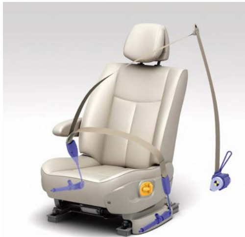
Figure 42: Drivers seat with seatbelt. The seatbelt pretensioner can either be mounted on the retractor, the seatbelt buckle or the lap belt anchor. In this case a pretensioner is mounted on the lap belt anchor and the seatbelt buckle. (Courtesy of Renault)
