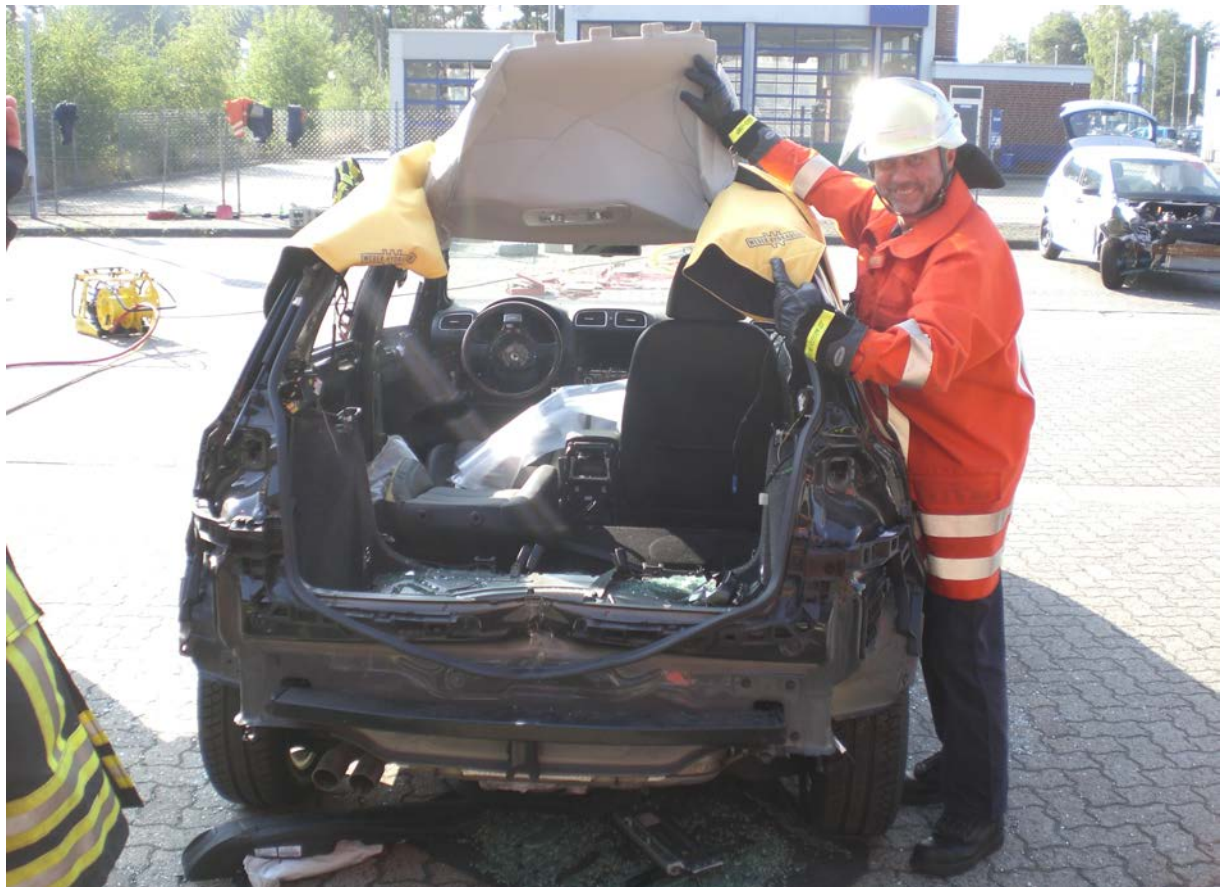
Figure 38: The sheet metal roof of this Volkswagen Golf has been cut on both sides with a reciprocating saw. Following the cuts it has been flapped forward together with the headliner. This allows enough space to extricate the driver to the rear of the vehicle.
