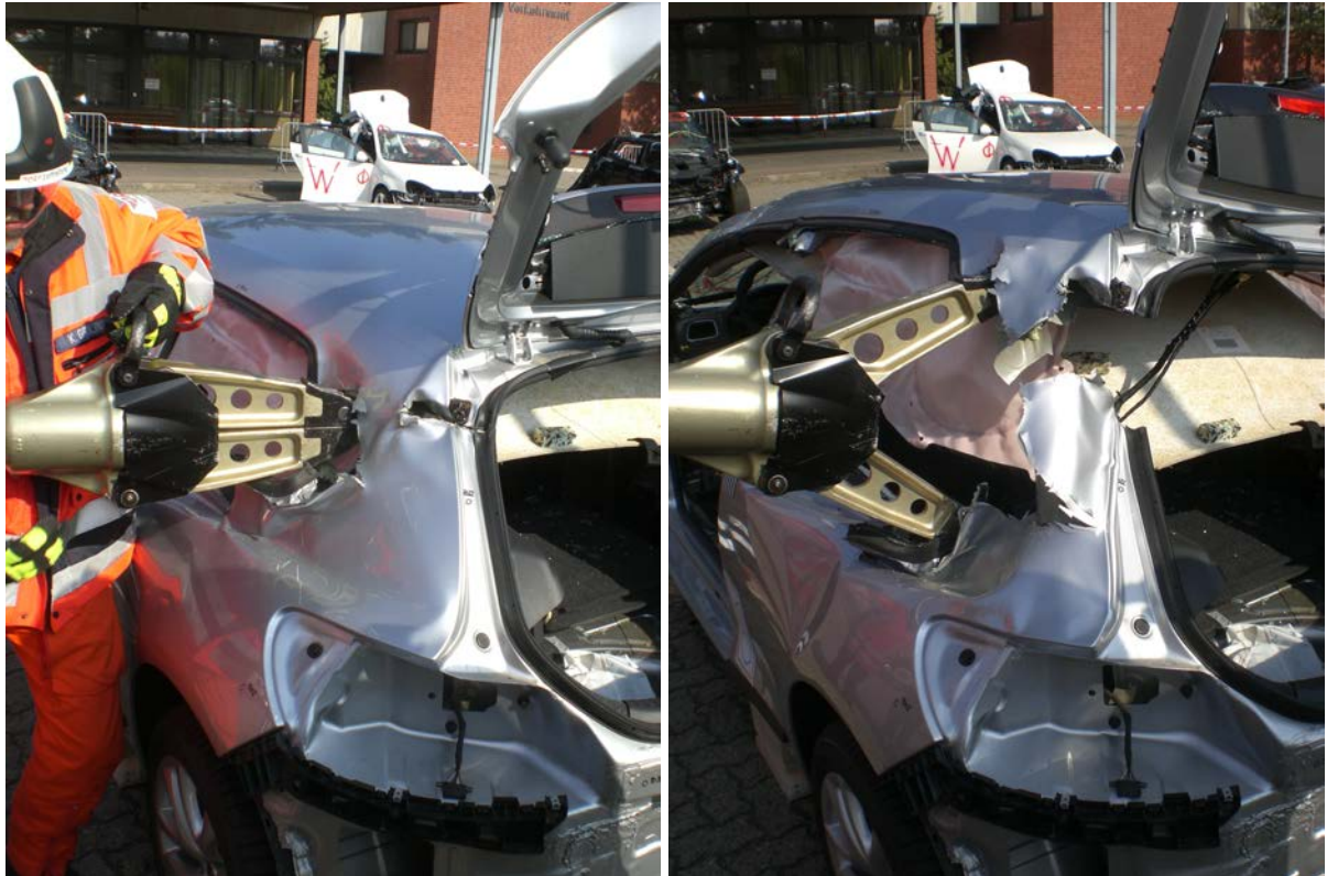
Figure 34: The spreader is utilized to rip the C-post of this Volkswagen Sirocco. Initially the tool operator unsuccessfully tried to completely cut the C-post with a cut from the left and from the right. Instead of trying to connect the two cuts he then utilized the spreader to rip through the remaining part of the roof post instead of trying to cut the remaining part of the roof post.
