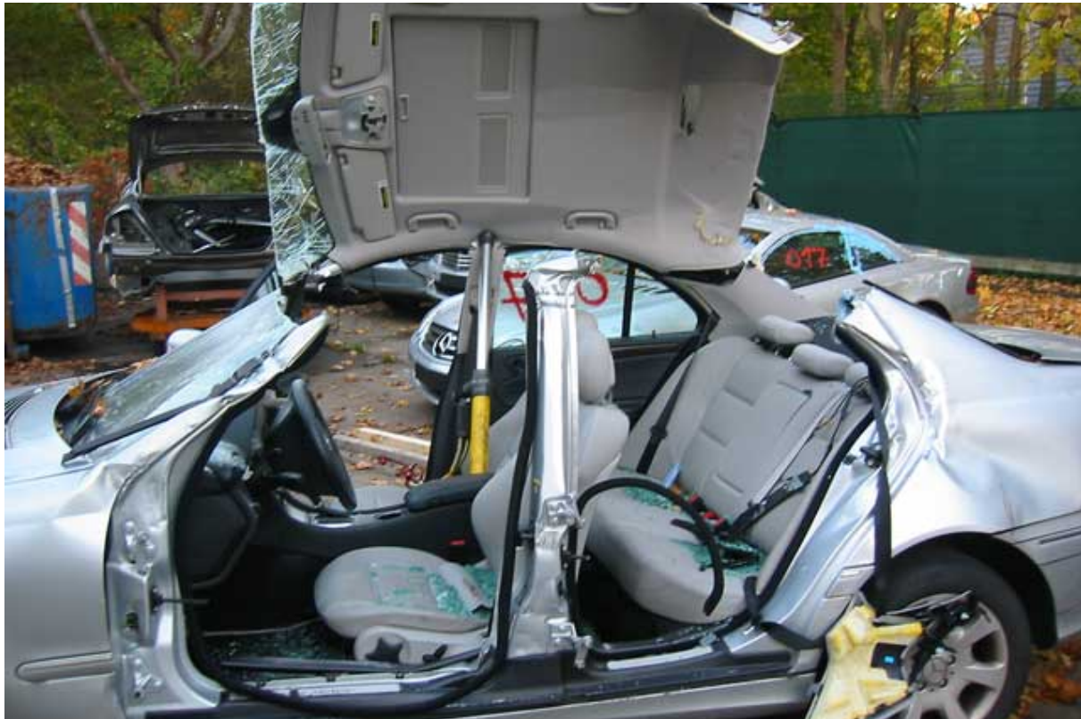
Figure 37: The roof of this Mercedes-Benz C-Class has been pushed out of the way instead of being removed completely, allowing to extricate the victim through the rear of the vehicle. This technique works best on vehicles with three roof posts. When force is applied on the center post on the uncut side, the roof will rotate upwards.
