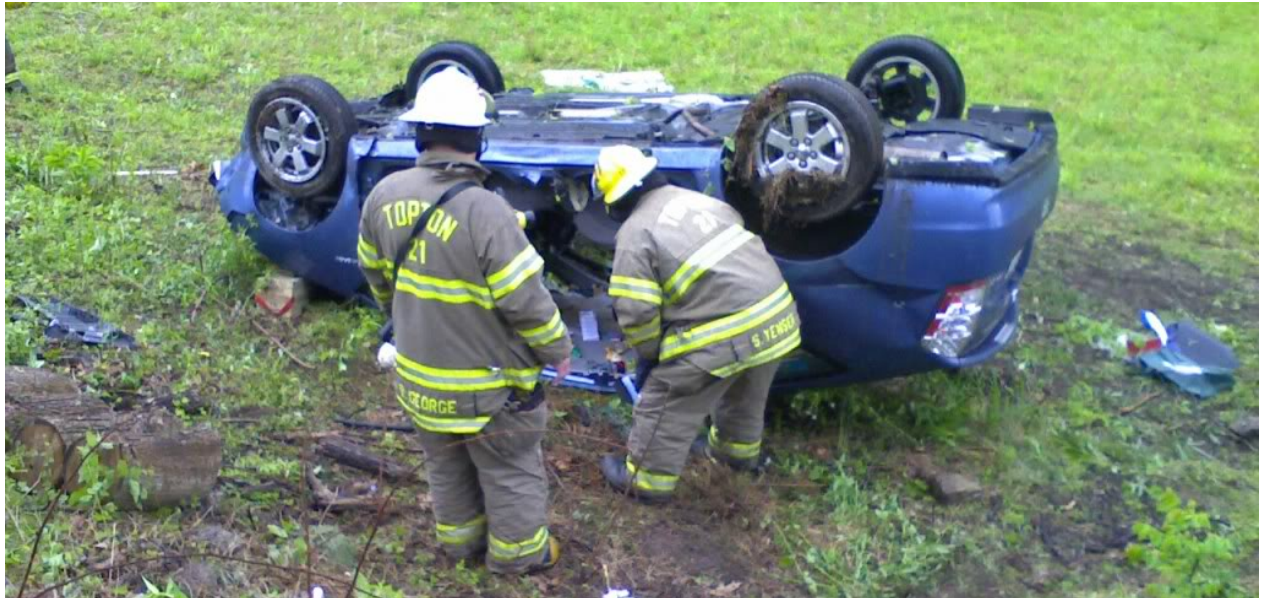
Figure 50: This Toyota Prius has been involved in a rollover crash. No airbags have been deployed. Emergency responders should take action to manually disable the vehicle. It is important in such a case to switch off the vehicle's ignition and to disconnect the 12 Volt battery which is located in the trunk of the vehicle and easily accessible in this case. (Courtesy of Tipton Volunteer Fire Company)
