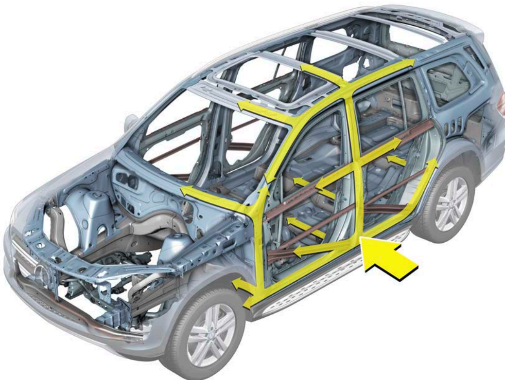
Figure 12: Body structure of a Mercedes-Benz GL-Class. The arrows indicate the load paths in case of a side collision. Unlike frontal collisions the distance between the occupant and the side structure is limited. Therefore there is no real crumple zone to absorb energy. The car
