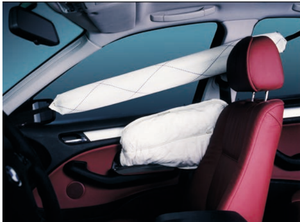
Figure 15: Door-mounted side airbag combined with an ITS (Inflatable Tubular Structure) head impact airbag. (Courtesy of BMW)
