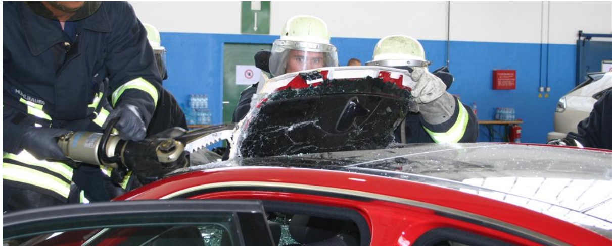
Figure 36: A hydraulic cutter is used to extend the rear window opening by creating a 'roof spoiler'. Cutting through the rear roof edge on the left and on the right side may allow to bend the center part of the roof forward and may already gain enough space to extricate an occupant through the rear window.
