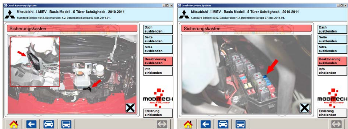
Figure 5: If the ignition key of this Mitsubishi i-MiEV (Electric vehicle) is not accessible, a certain fuse from the fuse box needs to be removed and the 12 Volt battery needs to be disconnected to completely disable the propulsion system.
