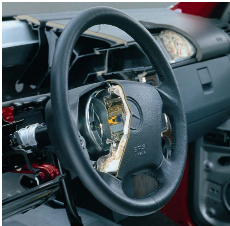
Figure 40: Cutaway model of a driver airbag. The pyrotechnic inflator is visible in the center of the steering wheel. Once ignited, the pyrotechnic charge will produce a large amount of nitrogen gas to fill the airbag in a couple of milliseconds. The inflating bag tears open the cover and expand to its maximum volume. (Courtesy of Daimler)
