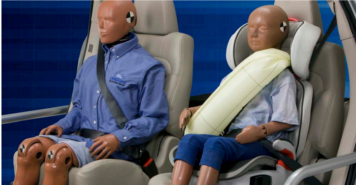
Figure 11: Inflatable seatbelt (belt-airbag) shown on the rear-seat occupants. The inflatable seatbelt distributes crash force energy better across the occupant's body. (Courtesy of Ford)
