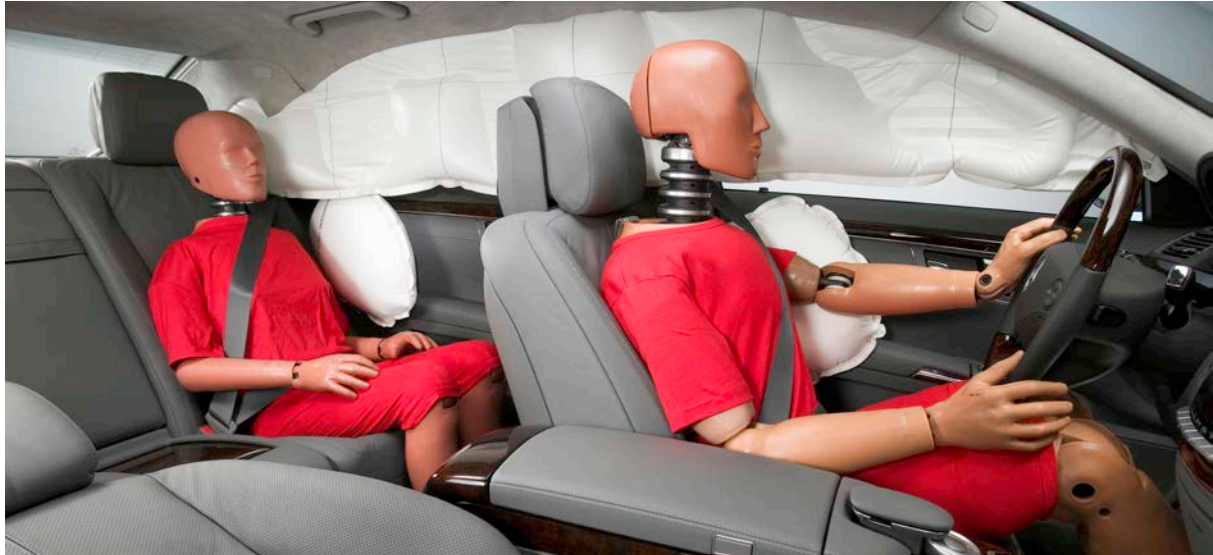
Figure 13: Seat-mounted side airbags for front and rear seat passengers are shown on this photo along with the curtain airbag deploying from the roof rail of the vehicle. (Courtesy of Daimler)
