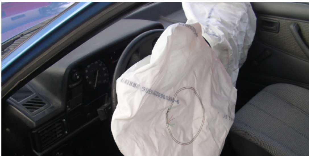
Figure 10: Simulated deployed driver and passenger airbags
