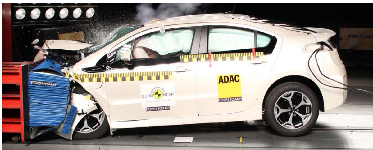
Figure 45: Moderate overlap crash test of an Opel Ampera. The test revealed that all safety features worked as planned. The propulsion system has been shut down on accident detection; the high-voltage battery has not been affected by the crash. (Courtesy of EuroNCAP)
