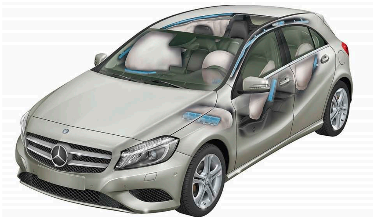
Figure 41: Airbag equipment of the Mercedes-Benz A-Class. A driver airbag, a driver knee airbag, a passenger airbag as well as front and rear seat-mounted side airbags are visible along the curtain airbags in the roofline. (Courtesy of Daimler)
