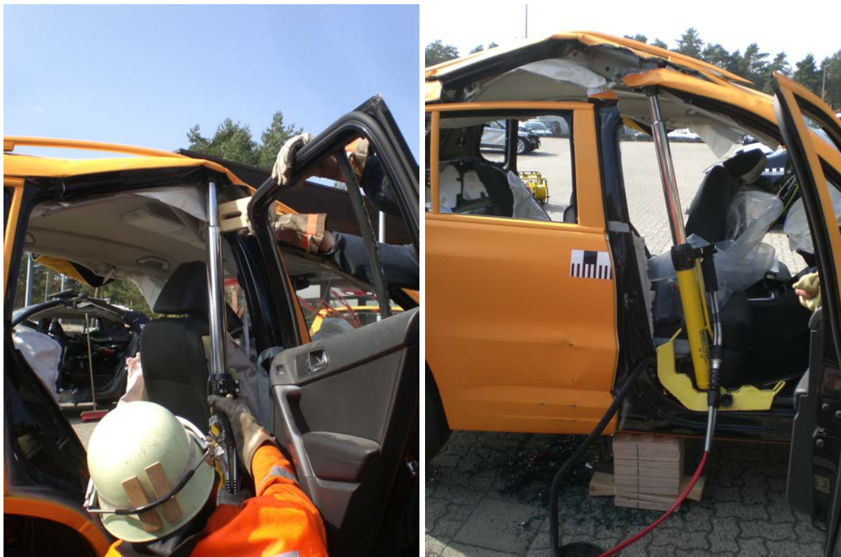
Figure 33: A telescopic ram is used to “ram” the roof of the B-post on this Volkswagen Tiguan. The initial push is performed behind the roof post. Note the wooden wedge that is used to protect the piston of the ram from being damaged by the ripped metal. After repositioning the ram to the front of the pillar the roof could be completely ripped off. Note the rocker panel support and the cribbing under the rocker panel to make sure the ram does not penetrate the rocker panel.
