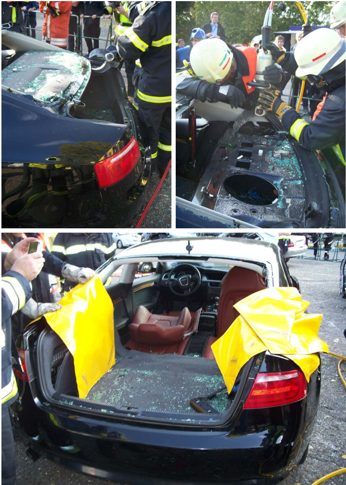
Figure 39: Tunneling through the trunk of an Audi S5. The rear hatch has been removed with a hydraulic cutter. The speaker deck has then been cut out with a reciprocating saw and a hydraulic cutter. In a last step the rear seatback has been spread out of the vehicle.
