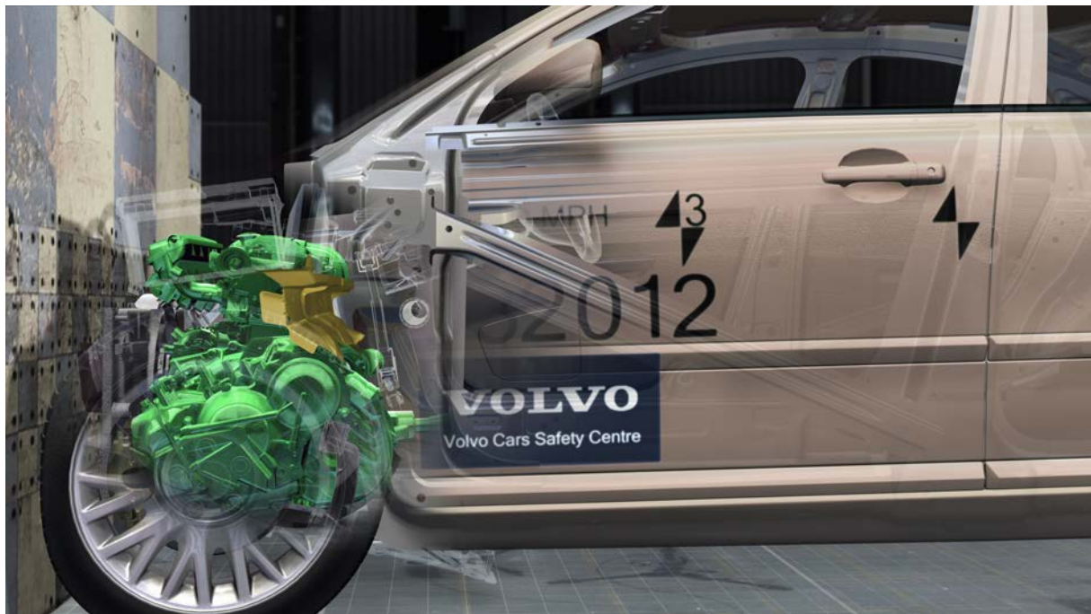
Figure 4: A cross member connecting both A-posts protects keeps the engine out of the passenger safety cell. (Courtesy of Volvo)
