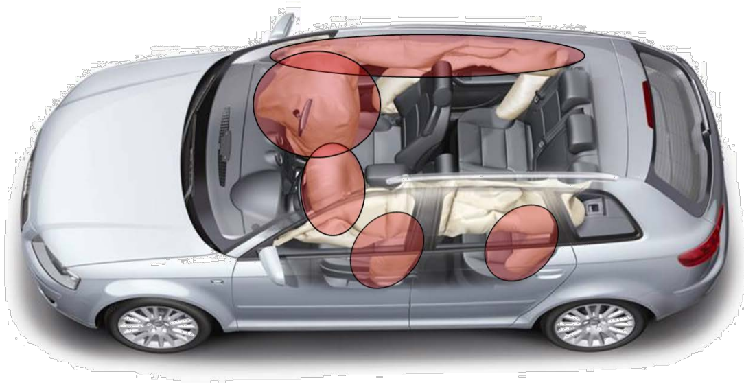
Figure 55: This graphic visualizes the necessary safety distances from any undeployed airbag. Emergency responders should stay 30 cm away from side and curtain airbags, 60 cm from the drivers airbag and 90 cm from the passenger airbag while working with rescue tool. (Courtesy of Audi)
