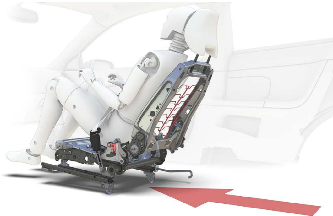
Figure 18: In Volvo's WHIPS (Whiplash Protection System) equipped seat, the entire seatback is designed to move together with the occupant in a rear-end collision. Therefore they are equipped with a piece of metal inside the seat that absorbs energy. (Courtesy of Volvo).
