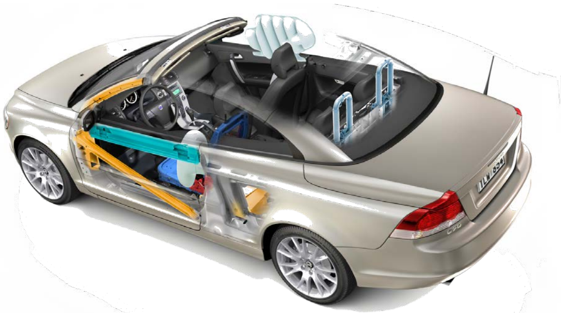
Figure 20: The safety system of convertibles has some special features. This images shows a door-mounted curtain airbag design as the curtain airbag cannot be stored in the retractable hard-top. The vehicle is also equipped with a rollover protection system behind the rear seats and a reinforced A-post. (Courtesy of Volvo)
