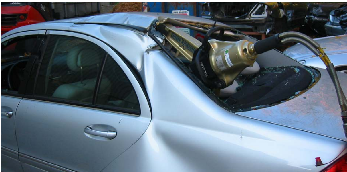
Figure 31: The photo shows an example of a method to quickly create a pathway for extrication through the rear window. Instead of totally or partially removing the roof of the vehicle the rear window opening can be widened with the spreader by either pushing the roof up or the speaker deck down.
