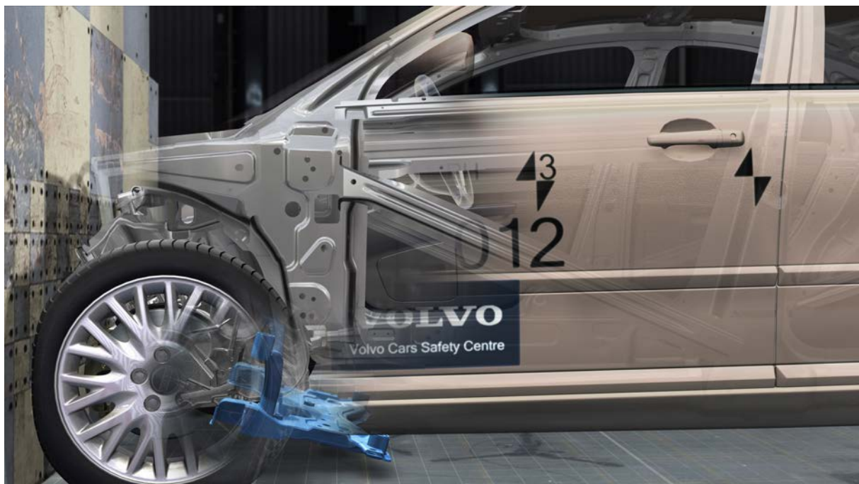
Figure 5: The wheels are pushed against and supported by the strong A-post to maintain the integrity of the footwell area. (Courtesy of Volvo)
