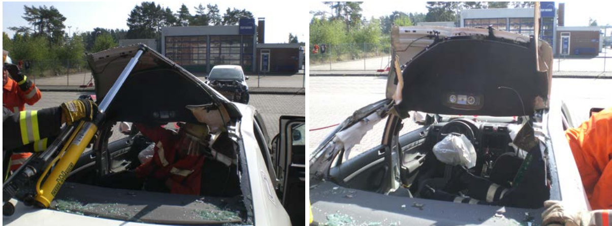
Figure 35: The rear portion of the roof sheet metal has been lifted with a hydraulic ram. Initially it may be necessary to make a relief cut at the left and right edge of the roof to define a starting point. Note that the roof has been ripped off at the weld spots where it has been attached to the roof rail.
