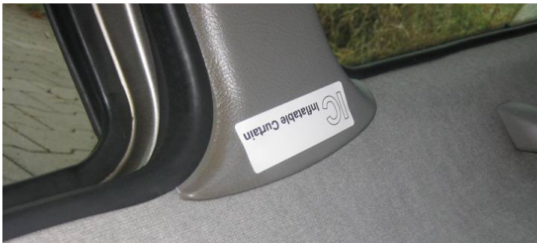
Figure 9: Simulated airbag label on the upper part of a B-post
