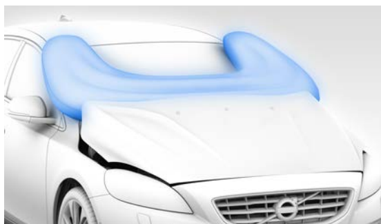
Figure 22: Pedestrian airbag shown on a Volvo V40. If a collision with a pedestrian is detected the hood hinges will be released by firing two pyrotechnic charges. The pedestrian airbag will inflate, raising the hood approx. 10 cm in the process to help absorb some of the impact. The airbag covers the lower edge of the windshield and the A-pillars in order to reduce the severity of head injuries from impact with these structures. (Courtesy of Volvo)
