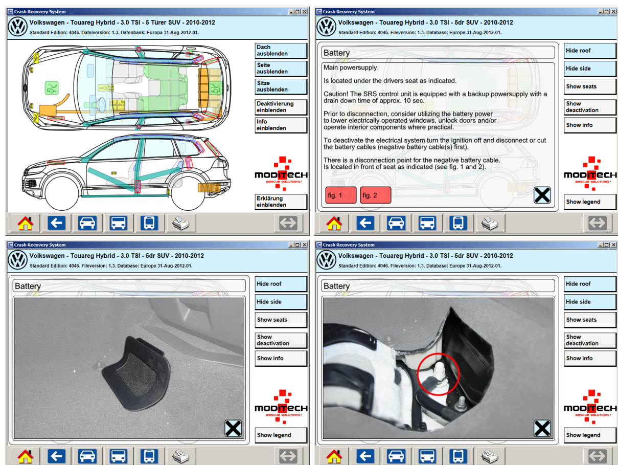
Figure 15: The 12 Volt battery of this Volkswagen Touareg Hybrid is located under the driver's seat. The negative battery cable can be disconnected from the vehicles body on the ground point in front of the driver's seat. This ground point is accessible through a flap in
